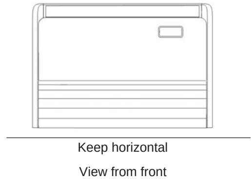
Fig. Inclination of Unit for Drain for wall mounted installation
